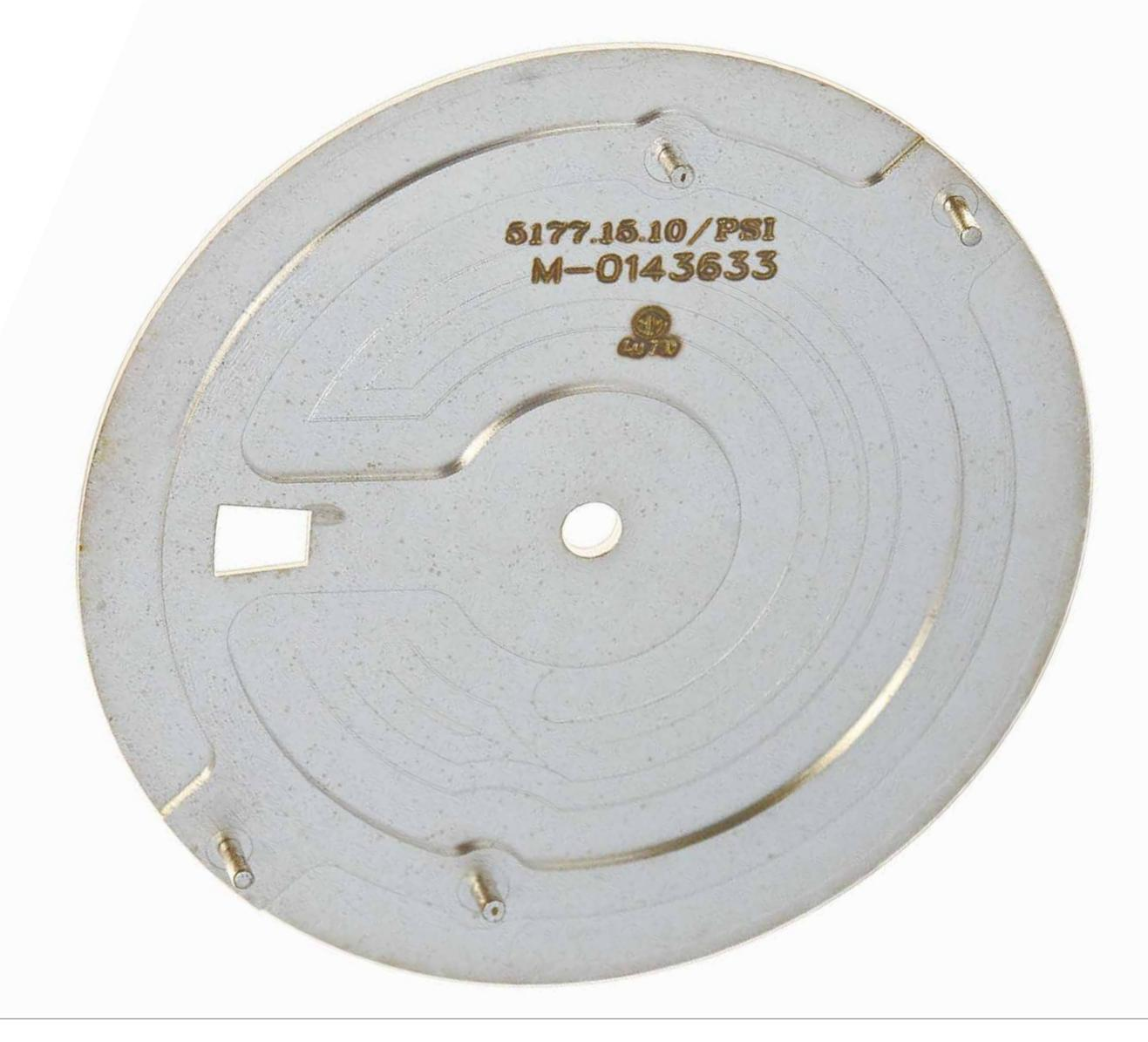
The dials are machined, including the dial feet, from a single disc of 18 carat gold. Four dial feet assure extra rigidity on the rose cutting engines when the dials are being cut, as well as security when sitting on the movement and movement ring. They are heavier than many conventional dials because of the density of the material and the large volume of the gold used.
